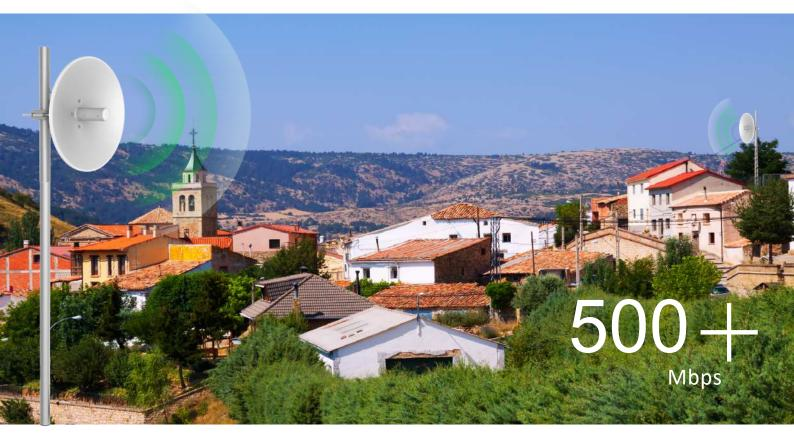
WIS-D525ACPro is a 500Mbps+ 2\*2MIMO Hi-Power outdoor wireless bridge based on 802.11a/n/ac technology. Featuring the revolutionary TDMA3 Intelligent Dynamic Polling Protocol technology, WIS-D525ACPro is fully compatible with WIS base station and bridge thus greatly improving the networks calability in throughput and latency.WIS-D525ACPro is best applied to rural wireless Internet,wireless backhaul and other industrial wireless surveillance solutions.
